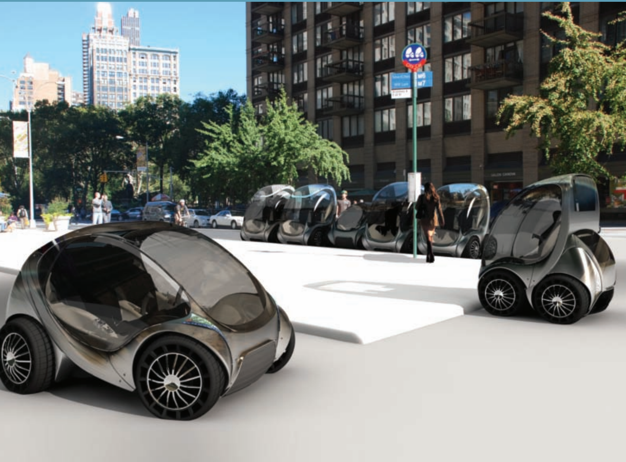
The CityCar, zooming into the future: This stackable electric vehicle gets the equivalent of 200 miles per gallon and is designed to be shared. William Lark, Jr., MIT Media Lab, Smart Cities
